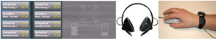
Fig. 3. From left to right: The dynamic priority list, the head-up-display, headphone based binaural auditory display and a wrist-watch attached tactile element
