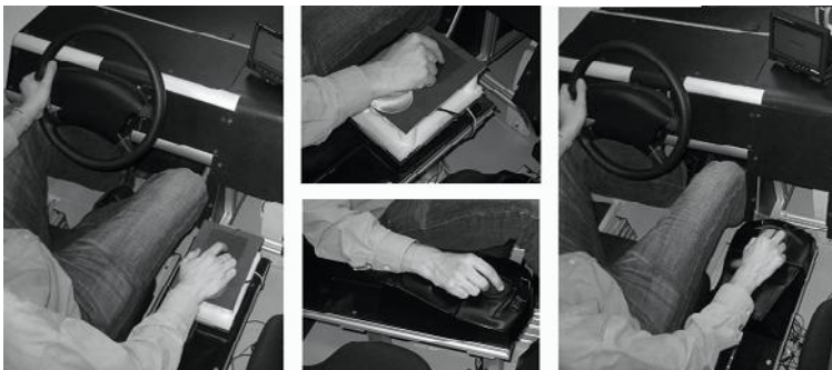
Fig. 2. Experimental setup with multimodal touchpad (left) and rotary push-button (right)
