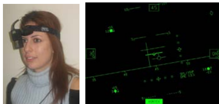
Fig. 8. The head mounted display and an example of the symbology of the HMD
